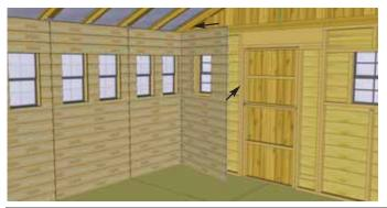
**20.** Locate Single Window Wall Panels (45" wide). All single window wall panels are built the same. Position in front corner. Slide edge tight in corner against side wall plywood backing. Adjust panel so window openings match. Secure with 6 - 1 1/4" screws. Complete each corner.
