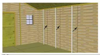
**39.** Locate Vertical Side Wall Trims. Position over seams in side walls on both sides of shed. Attach each piece with 6 - 1 1/2" Finishing Nails.
