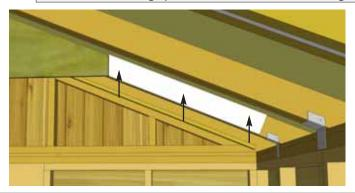
**4.** Locate Gusset Cleats (22.5 cut one end) and position on Rafter flush with Gusset. Attach Gusset Cleat to Rafter with **3 - 1 1/4" screws**. Complete remaining three Gusset Cleats.
