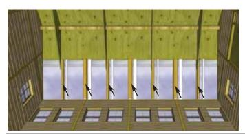
**40.** Attach Rafter Bottom Trims to cover underside of Rafters with Cedar Trim. Position under the Rafter and fasten with **5 - 1 1/2" Finishing Nails** per piece.
