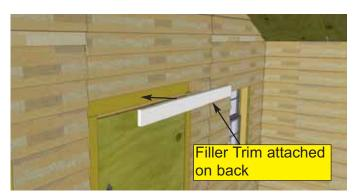
**35.** Locate Horizontal Door Trim and position on Door Header, tight against vertical Trim from the previous step. Horizontal trim will have an additional piece of wood pre-attached to the reverse face to make it sit flush to the wall. Attach trim with **3 - 1 1/2" Finishing Nails**.
