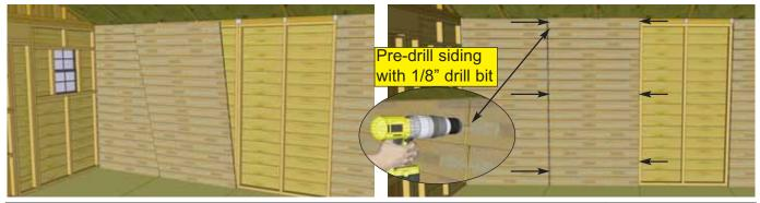
17. Locate Center Solid Wall Panel (45 1/4" wide). Center Wall Panels have siding flush with plywood backing. Position between previously installed panels and secure with 6 - 1 1/4" screws. Complete both center panels.
