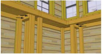
**45.** Position the Potting Shelves inside your Sunshed as desired, but the above configuration provides optimal sunlight exposure from the Polygal Roof and Windows. Attach the Shelves together with **2 - 2 1/2" Screws** to make them into a continuous Bench. You may also want to carefully screw the Bench to the wall in a couple concealed spots to keep it in place. Extra 2 1/2" Screws will be included in your hardware pack for this.
