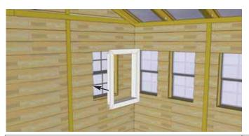
**42.** Locate the 4 large Window Inserts and position in window cavity. Nail to window wall framing with **9 - 1 1/2" Finishing Nails** from the bottom and sides. Complete the smaller window inserts in the same fashion.
