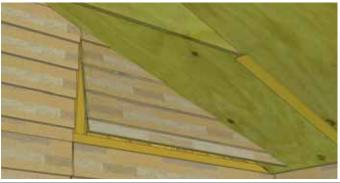
**25.** Locate Front Gable Panel Right and position in front corner of gable framing. Position and attach as per **Step 24**.
