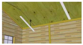
**41.** Locate Ceiling Trims and position over seam evenly to cover gaps between long ceiling panels. Attach each trim piece with **4 - 1 1/2" Finishing Nails**.
