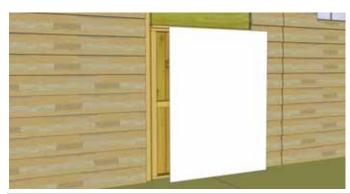
**30.** Position bottom door plywood on door. Position tight under new top cap and attach with **12 - 1 1/2" finishing nails**.
