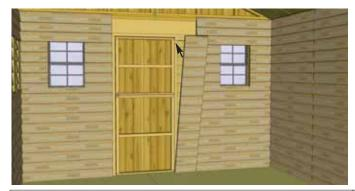
**22.** Position and attach Narrow Wall Panel next to door on wall framing. Attach with 6 - 1 1/4" screws.
