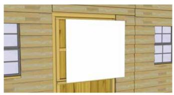
**29.** Position top door plywood over door framing. Confirm it is evenly spaced on door framing and attach with **12 - 1 1/2**" **finishing nails**.
