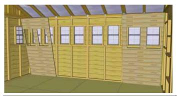
18. Locate Double Window Wall Panels Left & Right (42 3/4" wide). the panels have recessed siding as per Steps 15-16. Position on wall studs and secure as previously illustrated.
