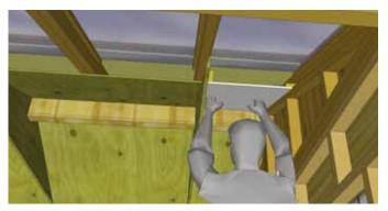
**12.** Locate and position rear ceiling plywood panel below Gable Ceiling Cleat and Short Roof Cleat. Attach panel to both Cleats with **8 - 1 1/4" screws**.
