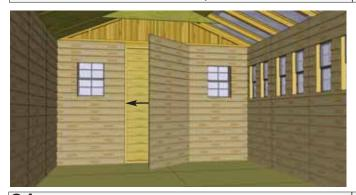
21. Locate Solid Center Wall Panel (45 1/4" wide). Center panel wall siding is flush with plywood backing. Position between previously installed panels on wall studs and secure with 6 - 1 1/4" screws.
