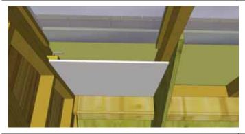
**9.** Locate and position front ceiling plywood panel below Rafter and Gable Cleat. Attach panel to Rafter and Gable Cleat with **8 - 1 1/4" screws**.
