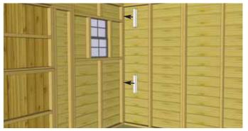
**14.** Position two Interior Wall Cleats against side wall in corner. Attach each Cleat with 2 - 2 1/2" screws. Attach cleats to each corner of your shed. Cleat provides an edge to screw Interior Wall Panel to in Step 15.
