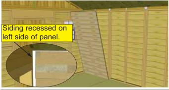
15. Locate Left Solid Wall Panel (42 3/4" wide). The left panel will have wall siding recessed on the left side as illustrated above. Position on wall studs and secure with 6 - 1 1/4" screws.
