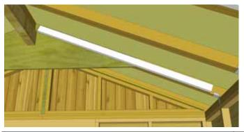
**5.** Locate Roof Cleats and position flush with Gusset and Gusset Cleat. Attach Roof Cleat to Gusset and Gusset Cleat with **4 - 2 1/2" screws** per cleat.
