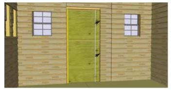
**32.** Position and attach the narrow wall door stop on framing with 6 - 1 1/2" finishing nails.
