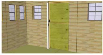
**31.** Locate all 3 door stops. Start on the door jamb side, position 2" wide stop against door jamb and the edge of wall siding. Attach with 4 - 1 1/4" screws.
