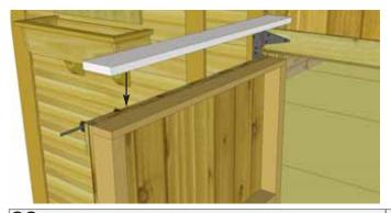
**28.** Position replacement top plate on bottom door and attach with **6 - 1 1/2" Finishing Nails**. Replacement Top Plate will cap door siding.
