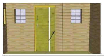
**34.** Locate Vertical Door Trim. Vertical Door Trim cover seams around the door and Narrow Wall. Position each piece over Narrow Wall Door Stop and wall seam. Attach each with **6 - 1 1/2" Finishing Nails**.
