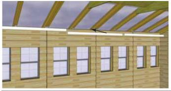
**38.** Locate Horizontal Side Wall Trims. Position trims up against wall siding and below ceiling plywood and Rafters. Evenly space trims on side walls and attach each piece with **4 - 1 1/2" Finishing Nails**.
