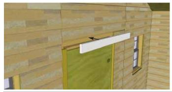
**33.** To complete the door stops, attach the Horizontal Door Stop against Door Header and attach with 3 - 1 1/4" screws.
