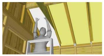
**6.** Locate long ceiling plywood (21" wide) and position up against rafter and ceiling gable cleat. Position squarely and attach with **12 - 1 1/4" screws.**
